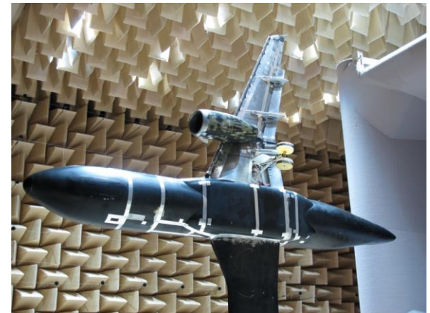
wind tunnel model in open test section of DNW-NWB
